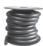
Fuel Line/Vapor Emission Hoses HBD Industries Nitrile tube hose is suitable with lead or unleaded gasoline and many Ethanol and Methanol-based gasohol blends. Meets or exceeds SAE30R7 specifications. This hose is not to be used for fuel injected systems.
